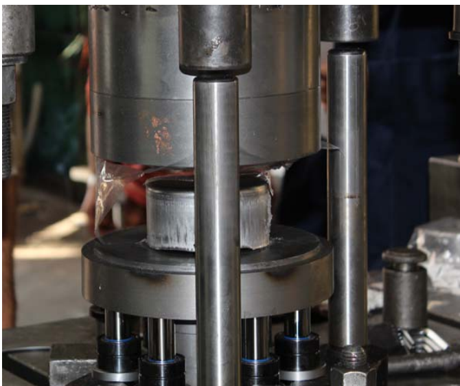
Figure 3. Deep drawing part obtained with film system
