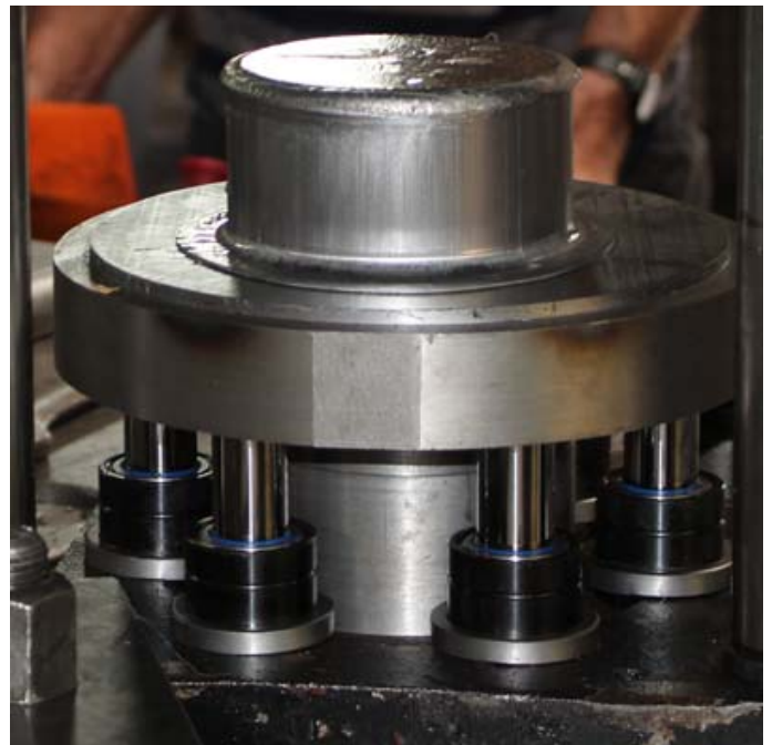
Figure 4. Deep drawing part obtained with lubricant system Deep drawing process parameters used in the study are presented in table 1.
